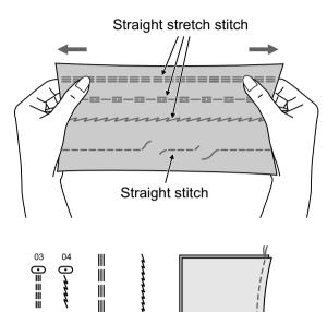
Use these stitches with knitted, tricot or other stretchy fabrics. The stitch enables your seam to stretch without breaking the thread.
