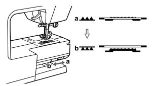
Sliding the lever to " **AAA** " (b) will lower the feed dog, for example during button sewing or monogramming. If you wish to continue sewing normally, slide the lever to "**AAA** " (a) in order to raise the feed dog.
