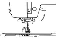
Lift the presser foot lifter to raise the presser foot bar.
