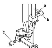
Remove the presser foot holder, and attach the darning foot to the presser foot holder bar.
