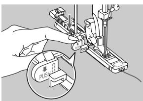
Pass the upper thread down through the hole in the presser foot.
