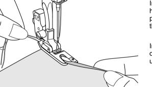
Insert the needle into the fold by rotating the handwheel toward you, and lower the presser foot. Sew several stitches and raise the presser foot.
