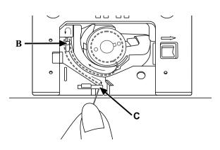
Pull the thread at the arrow markings into the stitch plate thread guide from (B) to (C). To cut off excess thread pull thread back over the cutting off blade at point (C). Close the bobbin cover plate.
