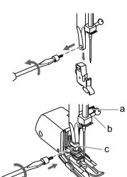
Remove the presser foot holder by unscrewing (counterclockwise) the presser bar attaching screw.
