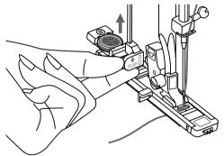
Raise the presser foot and cut the thread. To sew over the same buttonhole, raise the presser foot (it will return to its original position).
