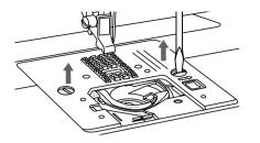
Remove the needle, presser foot and presser foot holder. Remove the screws holding the stitch plate and remove the stitch plate.
