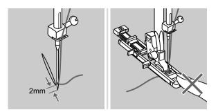
Position the fabric so that the needle is 2mm (1/16 inch) in front of the area to be darned. then lower the presser foot lever.
