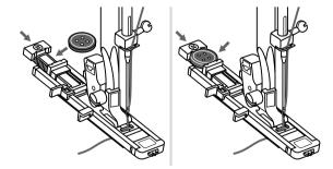
Attach the buttonhole foot, then pull out the button holder plate and insert the button.
