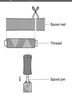
When using special threads which wind quickly off the thread spool, attach a net to the spool before using.
