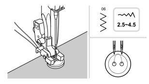
Position the work under the foot. Place the button in the desired position, lower the foot.
