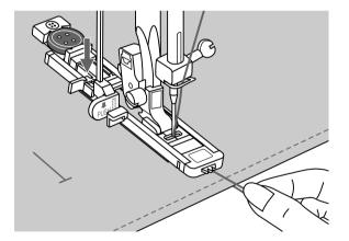
Slightly hold the end of the upper thread and start sewing.
