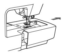
With the sewing table off the machine, the feed dog adjustment lever can be seen on the base at the rear side of the sewing machine.
