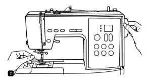
Hold the upper thread with the left hand. Turn the handwheel towards you (counterclockwise) lowering, then raising the needle.
