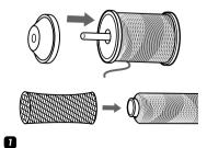
Lift up the spool pin. Place the spool of thread on the spool pin so that the thread comes from the left side of the spool, then place the spool cap at the end of the spool pin.
